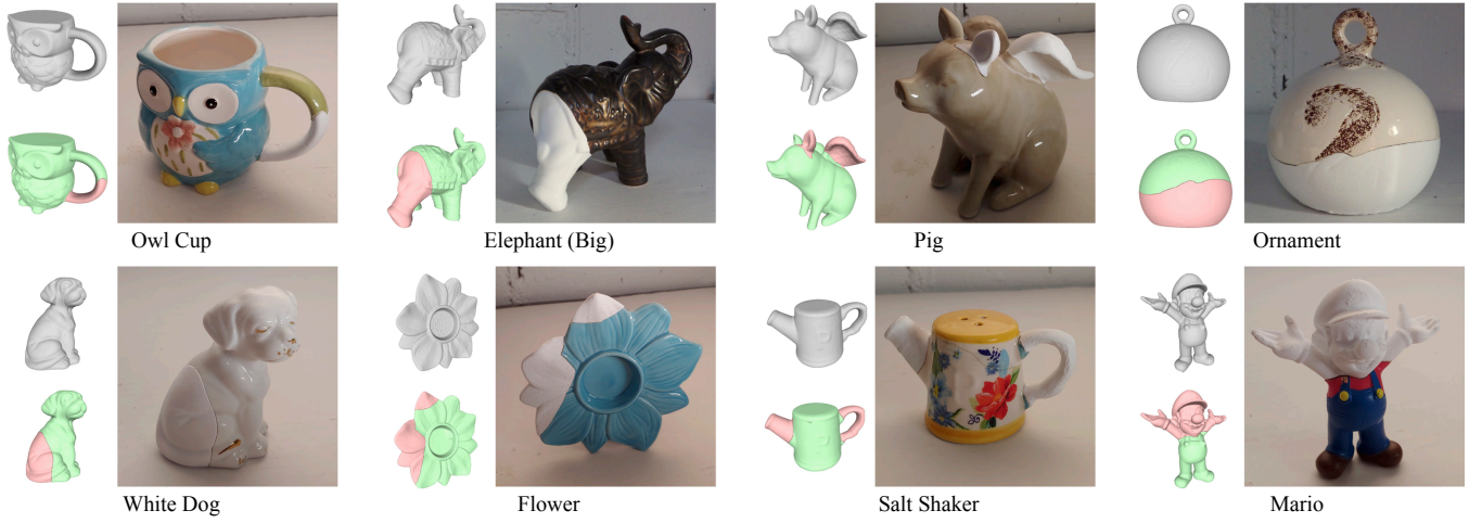
Figure 7: Original scanned mesh (gray), broken mesh (green) with restoration mesh (red), and 3D printed restoration piece joined to the broken piece for an owl cup, a big elephant, a pig, an ornament, a white dog, a flower, a watering can-shaped salt shaker, and a Mario figurine.
