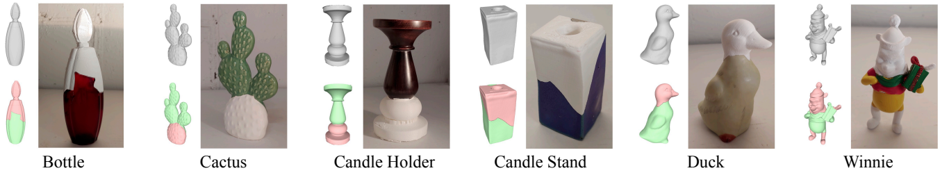
Figure 8: Original scanned mesh (gray), broken mesh (green) with restoration mesh (red), and 3D printed restoration piece joined to the broken piece for a bottle, a cactus, a candle holder, a candle stand, a duck, and a Winnie the Pooh figurine.
